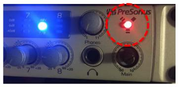
**STEP (4)** If it is red color, then PreSonus is not syncing with the host computer's FireWire. Power cycle the rack containing PreSonus, (or power cycle the PreSonus if not in a rack), and this LED should turn back to light steady blue color.
